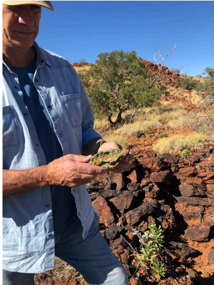
Figure 7: Nickel and copper-rich gossan outcropping adjacent to drill holes ADRC001 & 002
